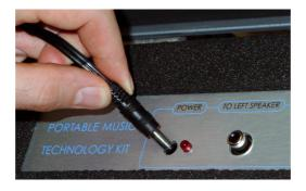
3. Connect the left hand speaker to the socket on the connection panel using the single phono cable with gold connectors.
