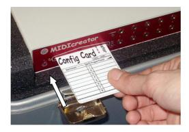
8. Insert the Smart Media Card into the slot in the front of the sampler (if required).
