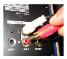
**Note:** Some kits are shipped with MA-10D digital speakers. If using these, please ensure you make connections to the sockets marked 'Line In' and 'Output'.
