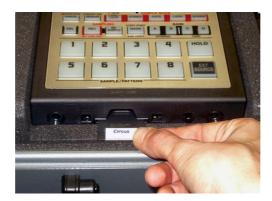
Whilst removing or inserting a card into the SP-303 sampler, hold down the 'Reset' button on the right hand side of the connection panel, above the sampler. This temporarily removes the power from the sampler, protecting the Smart Media card from damage.
