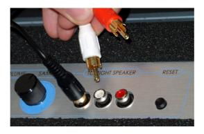
5. Connect the other end of the cable to the speaker. Ensure that the cables are connected to their corresponding coloured socket. Connect the power lead to the back of the speaker.
