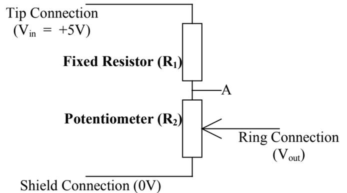
$$\text{Re-arranging equation (1) gives us : } R_1 = \left( \frac{V_{in}}{V_{out}} - 1 \right) R_2 = \left( \frac{5}{3.2} - 1 \right) 10K\Omega = 5.625 K\Omega$$
