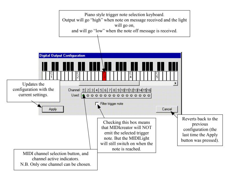
3. Select a MIDI channel. This determines which instrument you want to use and must be the same channel for both the upper and lower sockets that have the same note programmed into them i.e. the ones that will be linked together.
